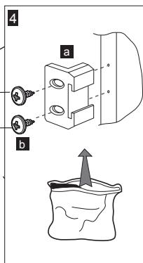
**Note:** Installation step for 2, screws for connecting top plastic part should not be screwed very hard, because of moving the plastic part easily left or right side. **Installation step for 4\* - only for Italy models.**
