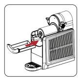
Install the condensation catch under the evaporator by sliding it into the rail grooves.
