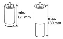
Oven height is 845 mm at minimum foot adjustment. Oven height is 900 mm at maximum foot adjustment.
