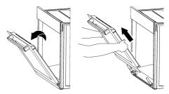
8. Pull the removed door upwards to release it from the right and left hinges and remove it.
