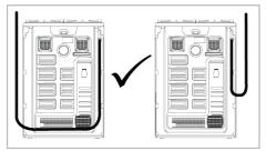
The gas hose should not be crushed, folded, pinched or come into contact with sharp corners or cookware utensils on the product. There is a risk of explosion due to damage to the gas hose!
