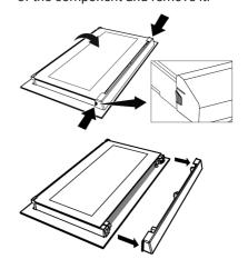
3. As shown in the figure, gently lift the innermost glass (1) towards "A" and then, remove it by pulling towards "B".
