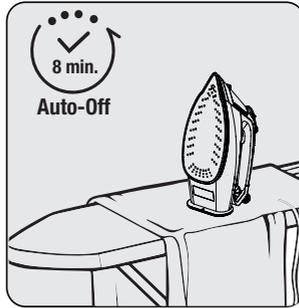
If you do not move the appliance for 8 minutes while in vertical position, it would shut-down automatically.
