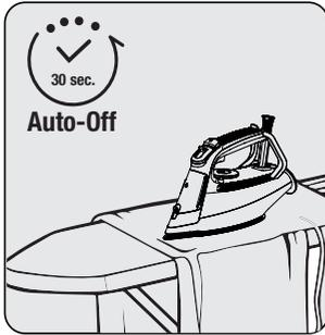
If you do not move the appliance for approximately 30 seconds while in horizontal position, it would shut-down automatically.
