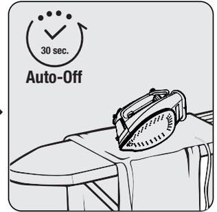
If you do not move the appliance for 30 seconds in lateral position (right or left), it would shut-down automatically.
