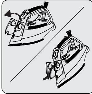
Open the water filling cap (2) and drain the remaining water in the water tank (8) by tilting the appliance forward.
