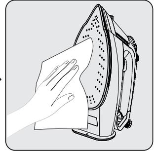
Wipe off any residues outside of the appliance and on the baseplate (9) using a damp cloth and, if necessary, a light, non-abrasive liquid cleaning agent.
