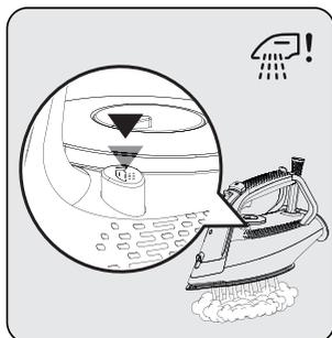
Place the appliance horizontally on the sink and shake the iron by pressing the "!" descaling button (7). Continue until the water in the water tank (8) runs out. When finished, release the descaling button (7).
