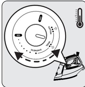
Set the appropriate temperature setting using the temperature adjustment button (6).
