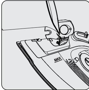
Fill the water up to the MAX line, holding the appliance in slightly vertical position.
