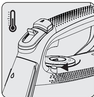
Set the temperature adjustment button (6) to the "MAX" position and wait until the thermostat light (10) turns off.
