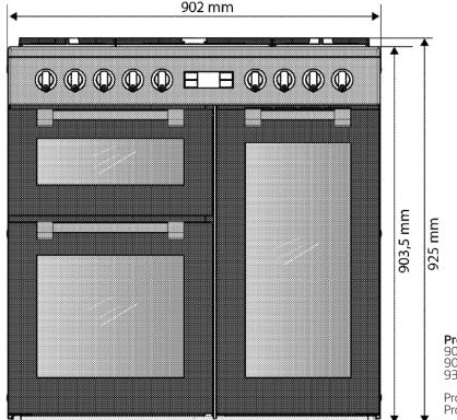
**Product Height** 900mm - without feet 903.5 mm - with feet fully tightened 930 mm - with feet fully open
