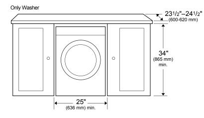
Required Minimum Clearances: (Stand Alone, Side by Side, or Stacked)
