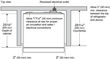
min. clearance between the top of refrigerator and alcove.
