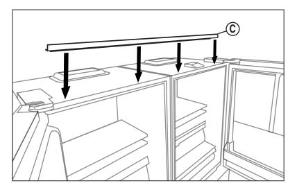
Open fridge doors. Dry fit L Angle Trim (C) on top of units. Make sure to have the outside of L Angle Trim (C) facing toward you. L Angle Trim (C) should be flush with front of fridge when doors are open.
