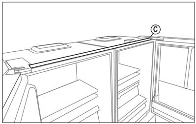
After making sure L Angle Trim (C) fits, peel film from Foam Tape on the bottom of L Angle Trim (C), and apply to the top of fridge units. Press fimly to adhear L Angle Trim (C) to fridge units.
