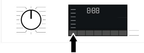
Whenever a new programme is selected, the recommended temperature for the programme appears on the temperature indicator. It is possible that the recommended temperature value is not the maximum temperature that can be selected for the current programme.
