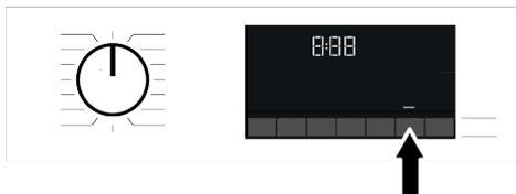
In order for the End Time function is activated and the programme is completed at the end of the specified time, you must press Start/Pause button after adjusting the time.
