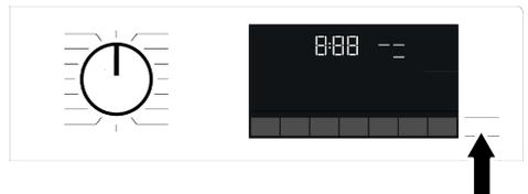
If the water level in the machine is not suitable when you press Start/Pause button, the door lock cannot be deactivated and the door lock symbol on the display remains on.
