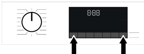
3. When the appliance is in HomeWhiz setup mode, you will see an animation on the display and the bluetooth icon will flash until your machine gets paired with smart device. Only programme knob will be active in this mode. Other buttons will be inactive.
