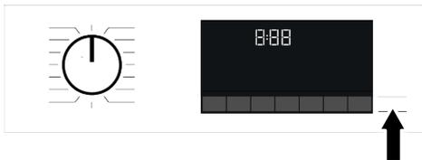
3. Loading door is locked. The door lock symbol appears on the display after the loading door is locked.
