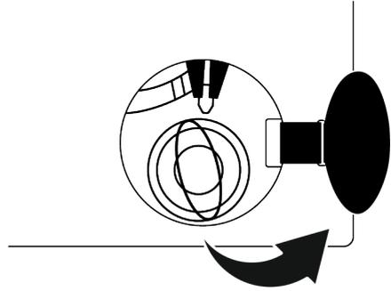
3. Pull down the loading door emergency handle with a tool and release. Then open the loading door.
