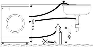
4. To prevent the waste water to go back into the product again and to ensure easy drainage, do not immerse the end of the hose into the waste water or do not insert it into the drain for more than 15 cm. If it is too long, cut it short.
