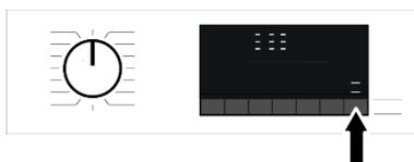
When the Remote Control is on, you can only manage, turn-off and status follow-up operations through your washing machine. And all functions except child lock can be managed through the application.
