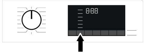
Whenever a new programme is selected, the recommended spin speed of the selected programme is displayed on the Spin Speed indicator. It is possible that the recommended spin speed value is not the maximum spin speed that can be selected for the current programme.
