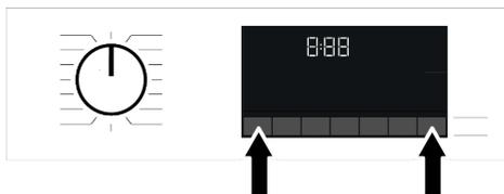
3. When in HomeWhiz setup mode, an animation appears on the screen and the Wireless Connection icon flashes until your machine connects to the internet. Only programme knob will be active in this mode. Other buttons will be inactive.
