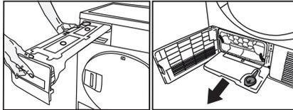
2. Drain the water in the tank.
