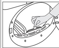
There are dampness sensors in the dryer that detect whether the laundry is dry or not. To clean the sensors:
