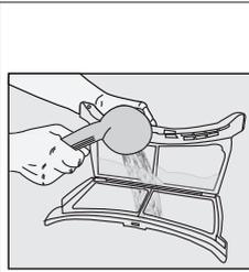
A layer can build up on the filter pores that can cause clogging of the filter after using the dryer for a while. Wash the lint filter with warm water to remove the layer that builds up on the lint filter surface. Dry the lint filter completely before reinstalling it.
