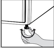
Turn the feet to left or right until the dryer stands level and firmly.
