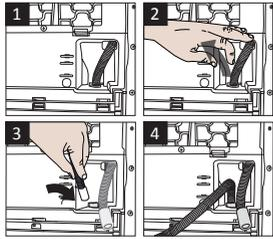
**1-2** Pull hose at the behind of the dryer by hand in order to disconnect it from where it is connected. Do not use any tools to remove the hose.
