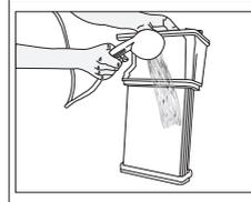
Clean the condenser by applying pressurized water with a shower armature and wait until the water drains.
