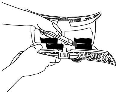
5. Clean both filters under running water in reverse direction of fiber accumulation with your hand or with a soft brush. Dry the filters before placing them back.
