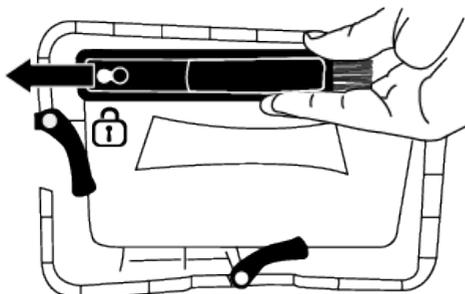
Clean the fiber on the metal surface of the condenser with damp cloth or with the brush on the air deflector in up - down direction. Do not clean in left - right direction since it will damage the metal plates of the condenser.
