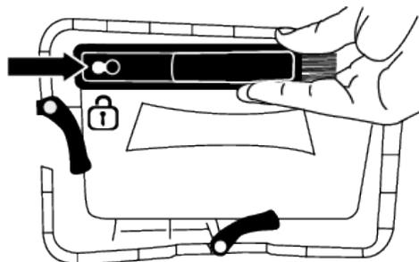
After the cleaning process is completed, place the air deflector cover to its place, close the latches by moving them and close the kickplate.
