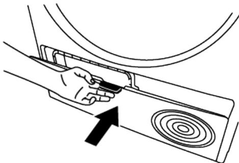
**NOTE:** You can clean by hand, provided you wear protective gloves. Do not try to clean with bare hands. The condenser fins may damage your hands. Cleaning from left to right may damage the condenser fins. This may lead to drying issues.
