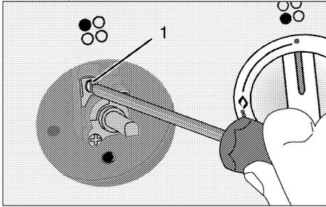
5. Set the flame length to 2 to 3 mm by means of the screw 1 on the oven tap. Turning in clockwise direction reduces the flame, turning counter-clockwise increases the flame.
