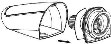
3. Remove the HEPA filter by grasping the handle of the filter holder and turning counter-clockwise.
