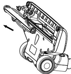
4. After cleaning and drying the roller brush, reattach it and lock the tab.
