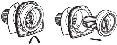
4. Wash out the dust container (10), filter holder and HEPA filter under the running water.
