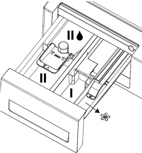
1) Left compartment with number "II" (Main wash compartment for powder detergent or powder bleach/stain remover)
