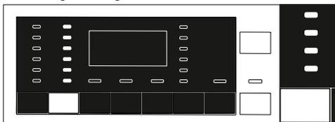
Whenever a new programme is selected, the spin speed recommended for the selected programme is displayed on the **Spin Speed** indicator.
