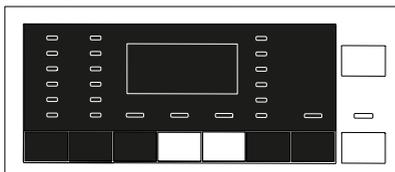
**Press and hold 2nd and 3rd auxiliary function buttons for 3 seconds.** After the countdown as "Child Lock 3-2-1" on the display is over, "Child Lock Enabled" appears on the display. You can release **2nd and 3rd Auxiliary Function** buttons when this warning is displayed.
