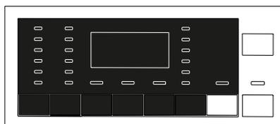
With the **End Time** function, the startup of the programme can be delayed up to 24 hours. After pressing **End Time** button, the programme's estimated ending time is displayed. If the **End Time** is adjusted, **End Time** light illuminates.
