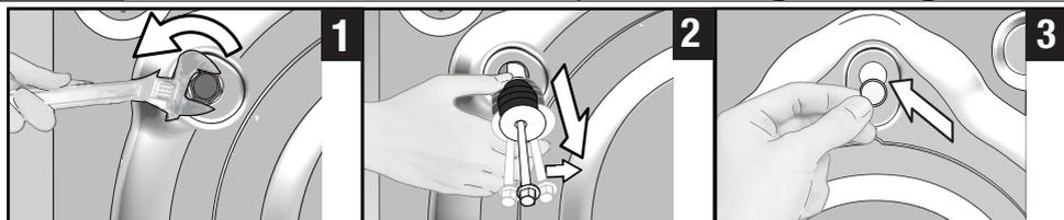
1 Use a tool to loosen all bolts until they rotate freely.
