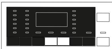
**Press and hold 2nd and 3rd auxiliary function buttons for 3 seconds.** After the countdown as "Child Lock 3-2-1" on the display is over, "Child Lock Enabled" is turned off on the display.
