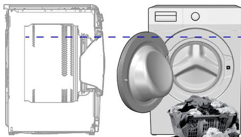
In 5 kg Wash & 5 kg Dry programme, it is recommended to load laundry until the level indicated in the above figure for ideal drying conditions (you will see the level arrow when you open the loading door).
