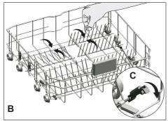
Finging the tines to the horizontal position by holding them from the tips may cause them to bend. Therefore, it will be appropriate to bring the tines in the middle to horizontal or vertical position by holding them from their stems and pushing in the direction of arrow.
