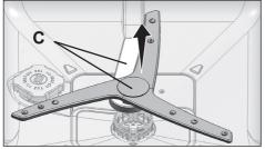
To remove and clean the lower impeller assembly together, hold by one hand from the (C) points shown in the figure and pull up to remove. After cleaning, follow these steps in reverse order to reinstall the impeller assembly.
