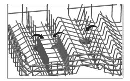
Bringing the wires to the horizontal position by holding them from the tips may cause them to bend. Therefore, hold the wires from their stems while bringing them to the horizontal or vertical positions.
