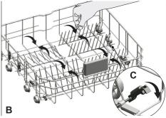
position by holding them from the tips may cause them to bend. Therefore, it will be appropriate to bring the tines in the middle to horizontal or vertical position by holding them from their stems and pushing in the direction of arrow.
