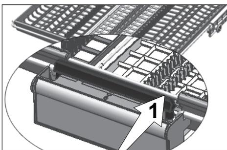
In models with partial movement feature, pushing the bar (1) on the handle enables the central tray of the basket to get to the lower position and the system gets unlocked. Thus right and left side trays can be used as moving parts. The free space enabled by the side trays allows long parts to be loaded in the upper basket.
