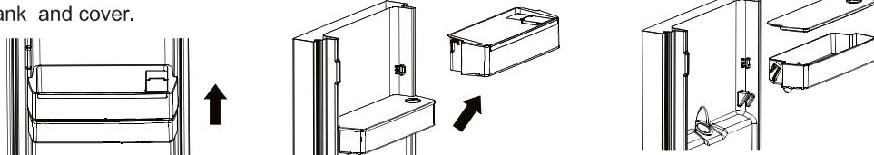
2. After cleaning, reposition water tank, cover and tank balcony as below process.
