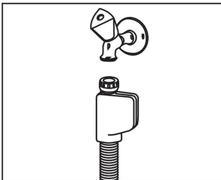
**⚠** As the hose set contains electrical connections and assemblies, never shorten or lengthen the hose with extension hoses.
