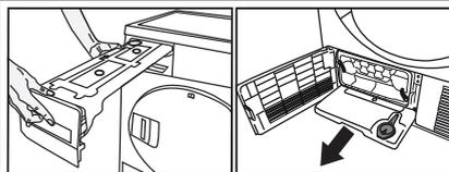
2. Drain the water in the tank.
