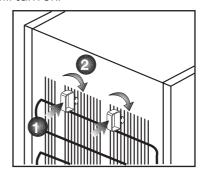
The condenser of your appliance is located on the back as shown below. In order to achieve better energy efficiency with lower energy consumption, please pull the condenser towards yourself as illustrated in picture below.
