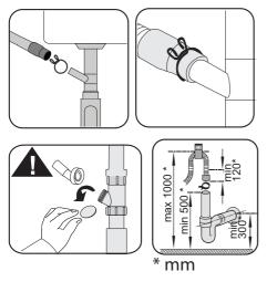
Drain pipe must be connected to the sewage system and it should not be connected to any surface water.
