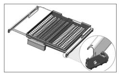
When the central tray is in the lower position, you can load long/high items such as coffee cups, ladles, etc. on the tray. When the side trays lean on two side walls, the handle can be pulled to allow the central tray to rise and the system to be locked.
