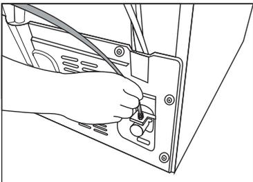
2. Connect the other end of the water hose to the water pump by pushing the hose into the pump's hose inlet.
