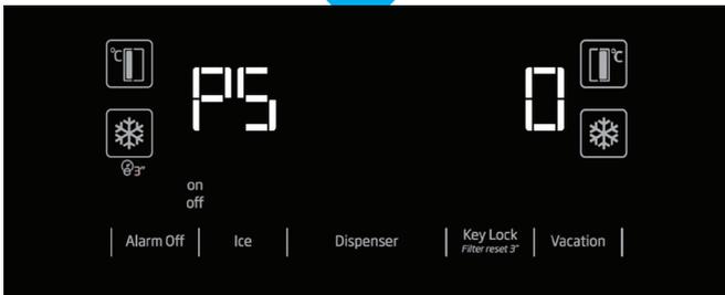
“Upon seeing PS 0 screen, de-energise the refrigerator and energise it again. This way, the filter counter will be activated. The filter warning LED will be active on the display in 130 days. After replacing the filter with a new one, press the Key Lock button for 3 seconds to make the filter counter to count down from 130 days. Repeat the steps given above to cancel this function.”
