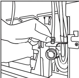
4. Connect the other end of the hose to the water mains (See Section 3.7) or, to use carboy, to the water pump (See Section 3.8).
