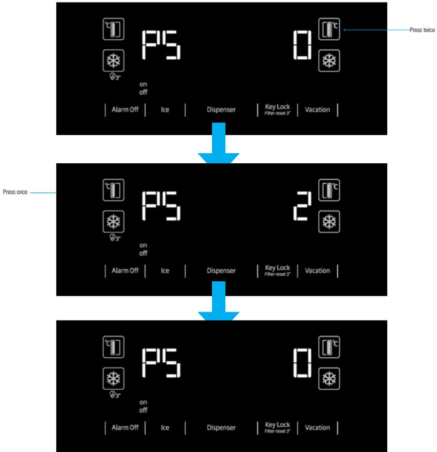
“Upon seeing PS 0 screen, de-energise the refrigerator and energise it again. This way, the filter counter will be activated. The filter warning LED will be active on the display in 130 days. After replacing the filter with a new one, press the Key Lock button for 3 seconds to make the filter counter to count down from 130 days. Repeat the steps given above to cancel this function.”
