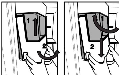
If you have difficulty in refitting the reservoir, turn the rotary gear 90° and reinstall it as shown in the figure 3. Any sound you hear when the ice drops into the reservoir is a part of normal operation.
