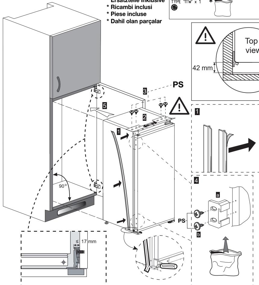
**Note:** Installation step for 2, screws for connecting top plastic part should not be screwed very hard, because of moving the plastic part easily left or right side.
