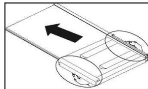
To remove the foldable wine rack, firstly, remove the glass shelf from the refrigerator. Then hold the plastic part and pull it to any sides direction. Now the product can be used without foldable wine rack if needed.
