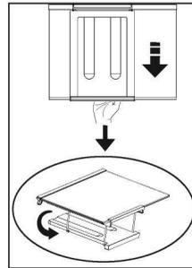
To assemble the foldable wine rack, firstly remove the glass shelf from the Refrigerator. Then hold the plastic part, and push it to any side direction by using plastic part's front and back areas . Now the product can be used with foldable wine rack if needed
