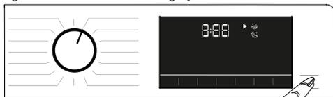
**If the water level in the machine is not suitable when you press Start/Pause** button, the door lock cannot be deactivated and the door lock icon on the display remains on.
