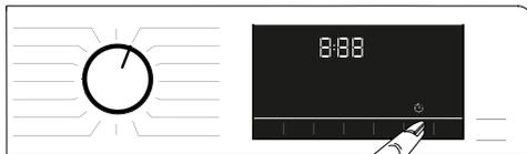
In order for the End Time function is activated and the programme is completed at the end of the specified time, you must press **Start/Pause** button after adjusting the time.
