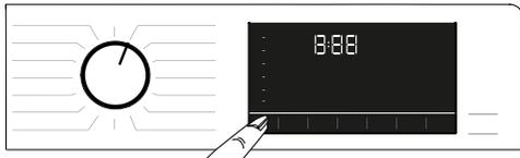
Whenever a new programme is selected, the recommended temperature for the programme appears on the temperature indicator. It is possible that the recommended temperature value is not the maximum temperature that can be selected for the current programme.
