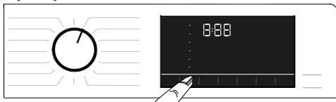
Whenever a new programme is selected, the recommended spin speed of the selected programme is displayed on the **Spin Speed** indicator.
