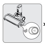
Push the roller release button to the left side.
