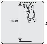
Position the charging dock at a height of minimum 112 cm from the ground.
