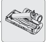
Fix the roller back to its place by pushing.
