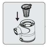
Attach pre-filter to the plastic filter back.
