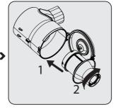
To insert the plastic filter, firstly place the plastic filter (1), then rotate it clockwise to lock it (2).
