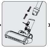
Press the electric turbo brush release button on the electric turbo brush and push it in the direction of arrow towards the tube.
