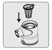
Attach pre-filter to the plastic filter back.
