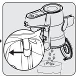
Pull the emptying dust container trigger to the last point. Dust container lid will be opened. Empty all the dust it contains.
