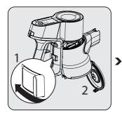
For a detailed cleaning of filters, remove the dust container by pushing the button to the left side.
