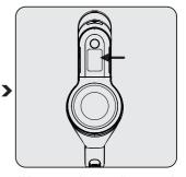
When you place appliance to the charging dock, it starts to charge and the battery charge percentage shall be displayed on the screen. Percentage (%) are increased as the appliance is charged.
