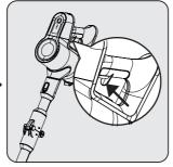
Press the on/off button to operate the appliance. The appliance starts operating with the minimum power when the on/off button is pressed.
