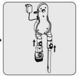
Attach crevice attachment and combination tool to the charging dock.
