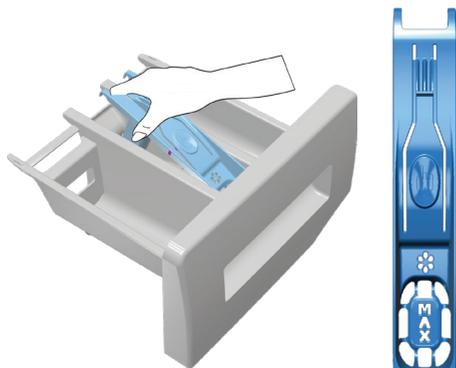
Lift the rear part of the siphon to remove it as illustrated.
