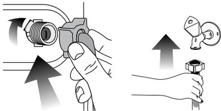
Open the taps completely after making the hose connection to check for water leaks at the connection points. If any leaks occur, turn off the tap and remove the nut. Retighten the nut carefully after checking the seal. To prevent water leakages and damages caused by them, keep the taps closed when the machine is not in use.
