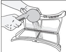
A layer can build up on the filter pores that can cause clogging of the filter after using the dryer for a while. Wash the lint filter with warm water to remove the layer that builds up on the lint filter surface. Dry the lint filter completely before reinstalling it.
