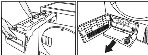
2. Drain the water in the tank.
