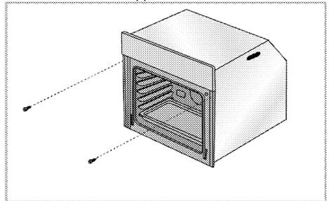
Secure the oven with 2 screws as illustrated.
