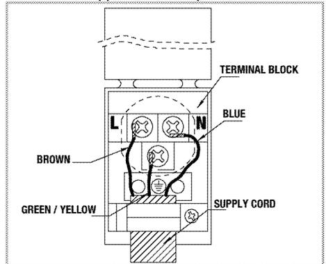
2. **For single-phase connection**, connect the wires as identified below:
