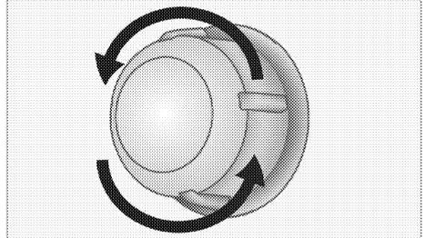
3. If your oven lamp is of type (A) shown in the figure below, remove it by rotating as shown and replace it. If it is of type (B), pull and remove it as shown in the figure and replace it.
