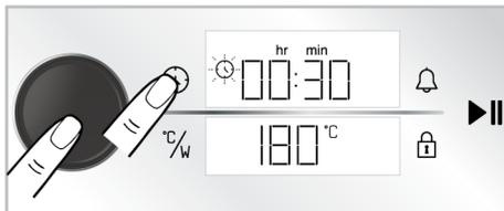
**i** To adjust the baking time quickly, you can activate the baking time as 30 minutes by pushing the oven control knob or touching the ⌚ key after the operation function and temperature are set, and you can change the time by turning the oven control knob to the right/left.
