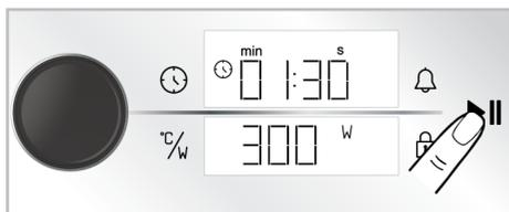
⇒ Your oven will start operating immediately in microwave function and power. The adjusted baking time starts to count down. On the display, the ► and W symbols are shown. When the baking time is completed, “End” text appears on the display, audible warning is given and baking stops.
