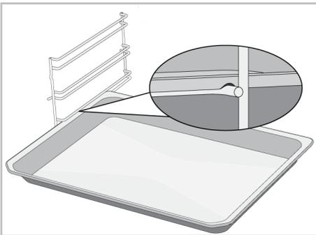
**Proper placement of the wire grill and tray on the telescopic rails-On models with wire shelves and telescopic models**
