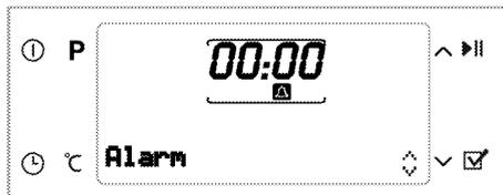
1. Press Time and Settings button (21) with short intervals until Alarm symbol (15) appears on the display.
