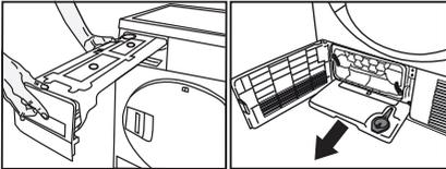
2. Drain the water in the tank.
