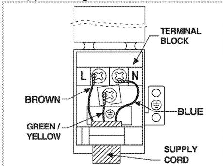
5. After completing the wire connections, close the terminal block cover.
