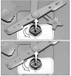
2 Pull out the metal/plastic filter (3) from the seating.
