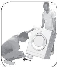
Tilt the machine backwards to remove the packaging reinforcement.
