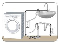
• Connect the drain hose to a minimum height of 40 cm and a maximum height of 100 cm.
