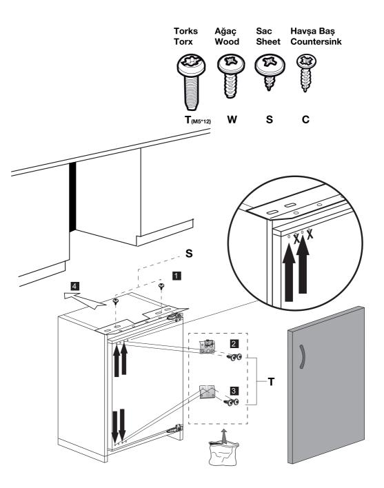
**Note:** Installation step for 2, screws for connecting top plastic rpart should not be screwed very hard, because of moving the plastic part easily left or right side.
