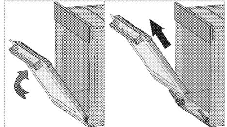
4. Remove the front door by pulling it upwards to release it from the right and left hinges.
