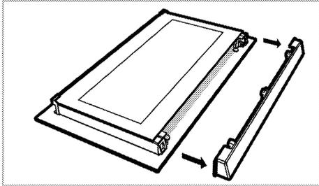
3. As illustrated in figure, raise the innermost glass panel (1) slightly in direction **A** and pull it out in direction **B**.
