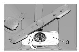
Press the two pawls on the coarse filter inwards and separate the coarse filter from the assembly.
