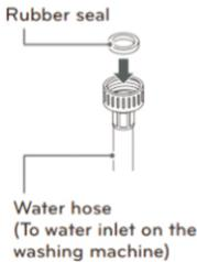
**2** Connect the water supply hoses to the water faucets tightly by hand and then tighten another 2/3 turn with pliers.
