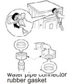
**The connection of inlet pipes and taps**
