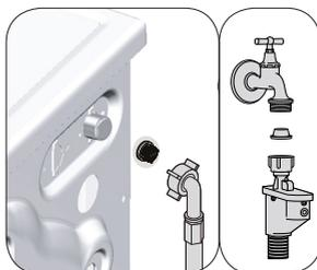
There is a filter at the end of each water intake valve at the rear of the machine and also at the end of each water intake hose where they are connected to the tap. These filters prevent foreign substances and dirt in the water to enter the washing machine. Filters should be cleaned if they are dirty.
