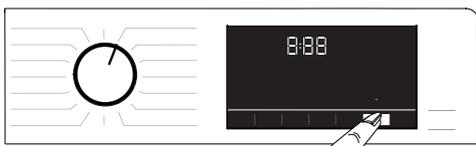
With the **End Time** function, start of the programme can be delayed up to 24 hours. After pressing the **End Time** button, the programme's estimated end time will be displayed. If an **End Time** is set, the **End Time** light will turn on.
