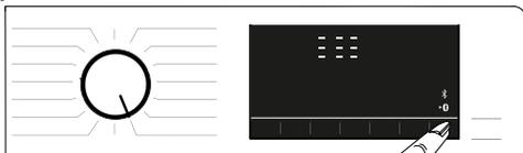
When Remote Control is enabled, you can only manage and switch off the machine and follow status on the washing machine.
