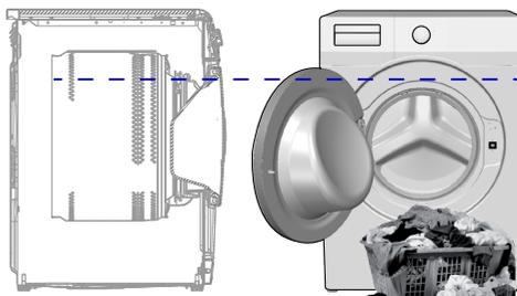
In the 4 kg Washing and 4 kg Drying programme, it is recommended to load the machine up to the level shown above for ideal drying conditions (you can see the level arrow if you open the loading door).
