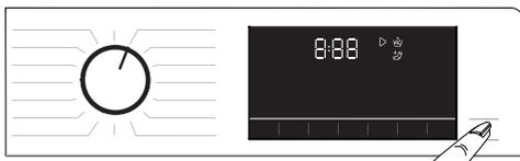
Press the **Start/Pause** button to switch the machine to pause mode.
