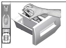
Clean the detergent drawer at regular intervals (every 4-5 washing cycles) as shown below in order to prevent accumulation of powder detergent in time.
