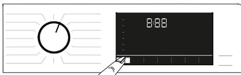
Whenever a new programme is selected, the temperature recommended for that programme appears on the temperature indicator. It is possible that the recommended temperature is not the highest value that can be selected for the relevant programme.
