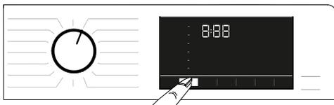
Whenever a new programme is selected, the spin speed recommended for the selected programme appears on the **Spin Speed** indicator.
