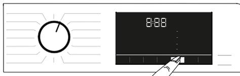
When you select a new washing programme, press the Auxiliary Function Selection button to set the drying option suitable for this programme.
