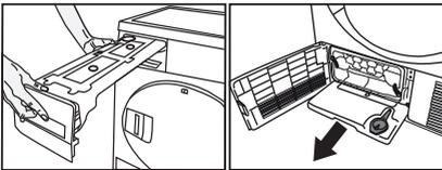
2. Drain the water in the tank.
