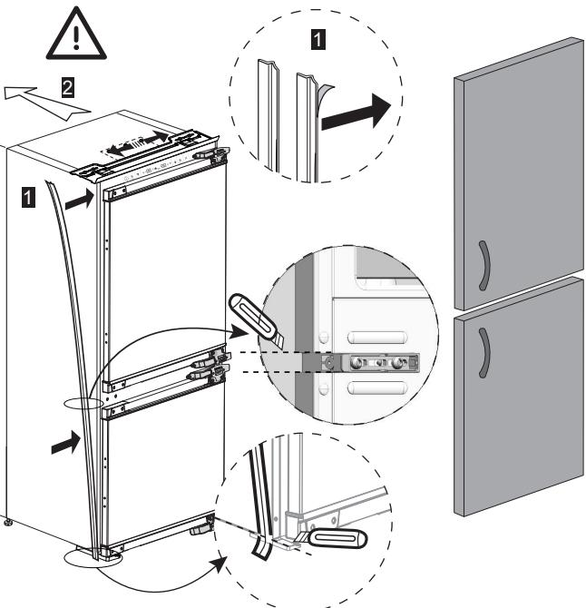
**Note:** Screws for connecting top plastic part should not be screwed very hard, because of moving the plastic part easily left or right side.
