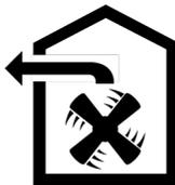
The air, which is sucked from the middle of the induction hob, passes through the oil filters and is discharged to the outside through the chimney with a pipe system.
