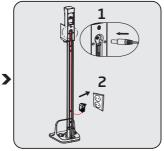
Install charging dock tube (16) to the charging dock support (17), then install the charging dock (15) to the charging dock tube (16). Install the thin end of the charger to the seat on the charging dock (15). Plug the charging adaptor (19) to the outlet.
