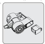
If you shall not be using the appliance for a long period of time, please keep the battery in a cool and dry place at half charged condition after removing it from the appliance. Do not charge or discharge completely.
