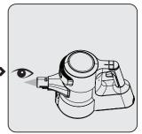
Inspect the vacuum nozzle of the appliance body (10). Remove any foreign materials.
