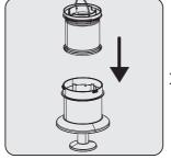
Install the dried inlet foam to the metal filter.
