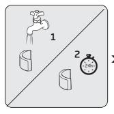
Inspect the outlet foam regularly. Clean it by washing under running cold water after removing the dust on them in case of excessive dust. Reinstall it once it is dried.
