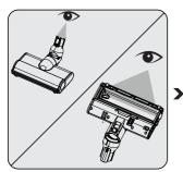
Inspect the connection point of the brush (8) and the vacuum nozzle. Remove any foreign materials.
