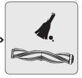
Remove the dust on it by tapping it lightly to a hard surface or remove the dust with a brush. If any hair, etc. is tangled, remove it by cutting it off.
