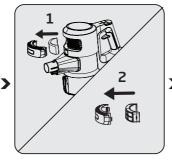
Remove the EPA E12 filter and the outlet foam inside it.
