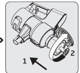
Install the metal filter and inlet foam inside the dust reservoir (11) by rotating the metal filter clockwise.
