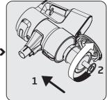
Install the metal filter and inlet foam inside the dust reservoir (11) by rotating the metal filter clockwise.
