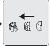
Install the EPA E12 filter and outlet foam to the lid.
