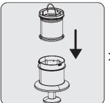
Install the inlet foam to the metal filter.
