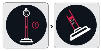
When the vacuum duct is blocked, the animation indicating that the duct is blocked is displayed on the screen continuously and the appliance stops operating. Determine the reason of the blockage of the vacuum duct.
