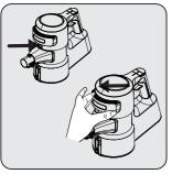
Remove the lid simultaneously while pressing the EPA E12 filter release button.
