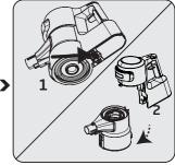
Push the trigger under the appliance to clean the dust reservoir (11).
