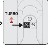
Press the "+" mode button (2) once to operate the appliance with medium speed. Press once more to operate it with the maximum speed.
