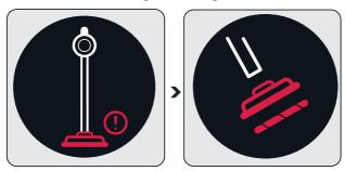
When the turbo brush is blocked or too many hair, etc. materials are tangled on the rotating roll, the animation indicating the brush blockage warning is displayed on the screen continuously and the appliance stops operating.
