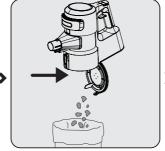
Press the dust reservoir lid opening button (12) to open the dust reservoir (11) and discharge the dust collected inside.
