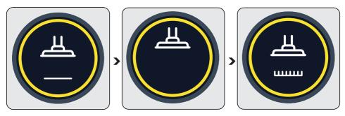
When the auto floor detecting brush (8) moves from a hard floor to a carpet floor, the figures shown above shall be animated on the screen (4).
