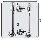
If you want to install the charging dock (15) to the wall, detach the charging unit from the tube (16) and support (17) using two separate buttons.
