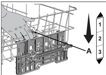
1. To raise the basket, hold the wires of the basket and pull the basket upwards with both hands while the basket is at the lowermost position (B)
